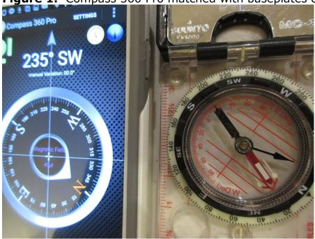
Figure 1 shows the app by itself, and another next to a mechanical compass, showing 235 and 233 degrees respectively, within plus-minus 2 degrees. --Brian Starlin
